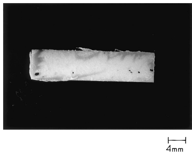
Fig. 10. Solidified molten surface textures of 6.1-mm-thick 30-GF-PBT specimens for a melt time of 15 s and a hot-tool temperatures of T_H = 230^\circ\text{C} .
